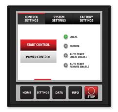
1 Set power control to Manual, Computer Interface, Watt Density or Proportional Speed Mode
