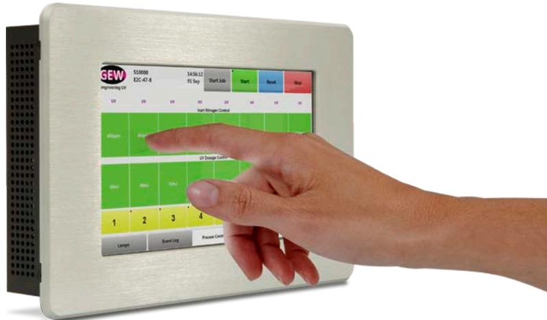
**Figure 38: Preparing to adjust Inert Gas Process Control parameters for lamp 2.**
