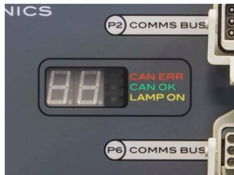
**Figure 11: The RPSU Front Panel Display**
