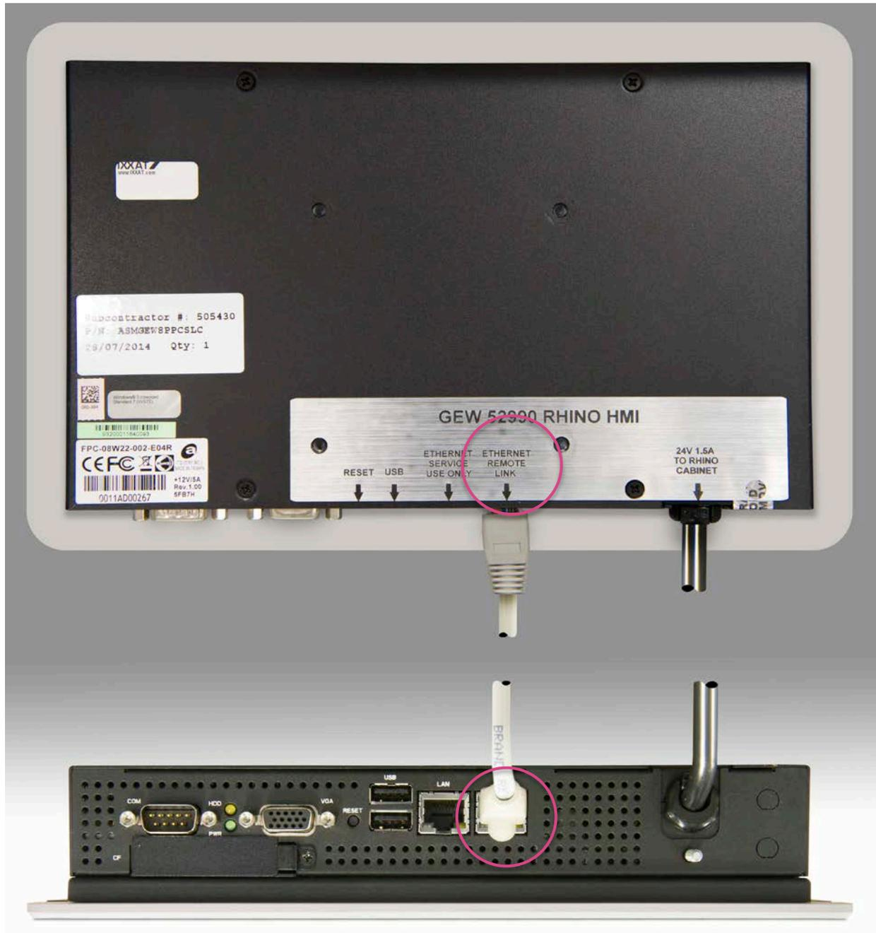
**Figure 24: Connections on the HMI**
