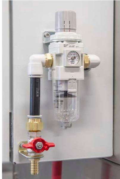
Figure 19: Inert gas pressure regulator and moisture trap
