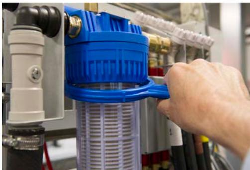
**Figure 10: Using the supplied wrench to remove the filter bowl**
