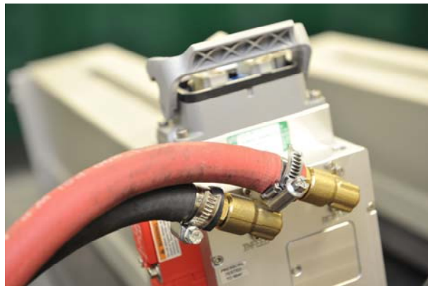
Figure 20: Typical water connections to lamphead
