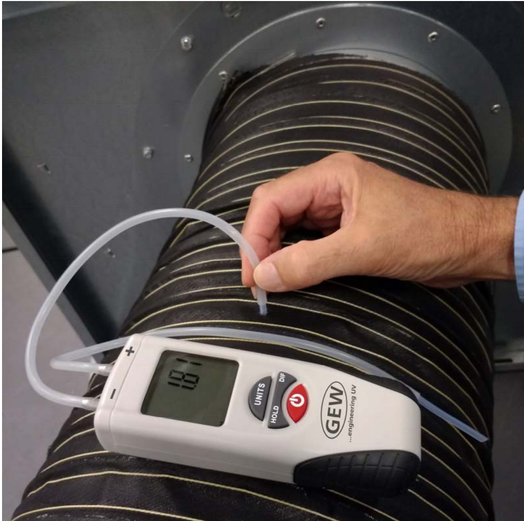
Figure 16: Taking a pressure reading using the manometer
