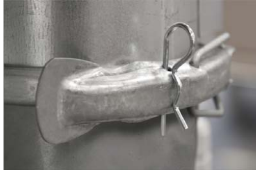
Figure 7: Locking pin fitted to clamp
