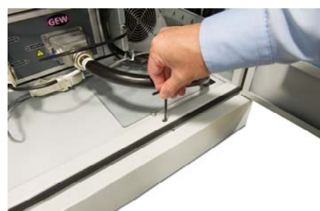
Figure 6: Removing RR lower panel for transport by forklift
