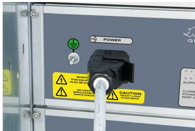
Figure 13: Power cable connection
