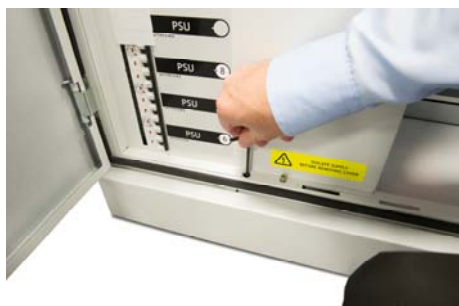
Figure 6: Removing RR lower panel for transport by forklift
