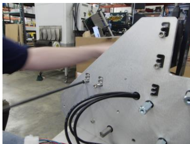
Figure 7: Remove top 2 screws on left panel to completely remove hold down assembly.
