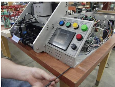
Figure 1: Remove control cabinet cover. Remove front panel.
