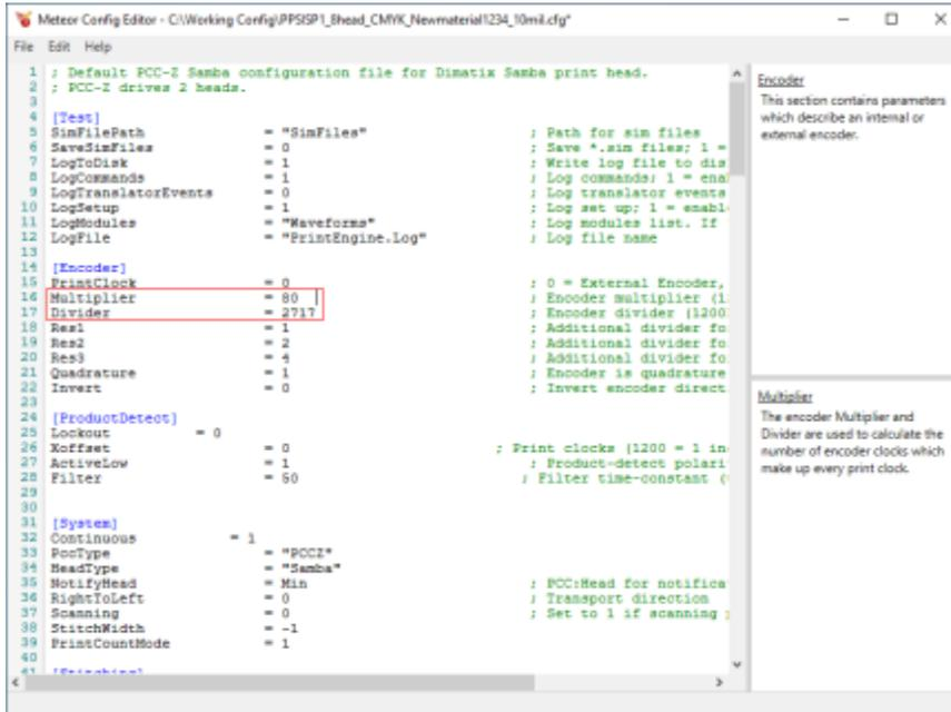
It is recommended to reprint the encoder line and remeasure to verify the results are correct. If these values are not correct, the process can be repeated to generate a new set of Multiplier and Divisor values.
