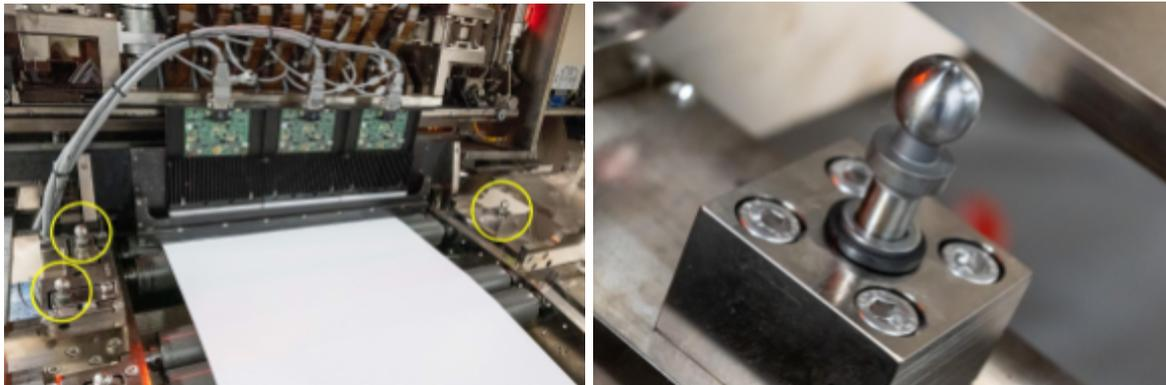
Next step is to verify the fly height is correct with the Stamp/Contact Test. This requires webbing up the new material and getting it under proper tension for printing. Once the material is correctly webbed and under tension, stop the press with the material still under proper tension.
